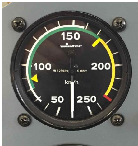
Figure 1 - Airspeed Indicator marking
