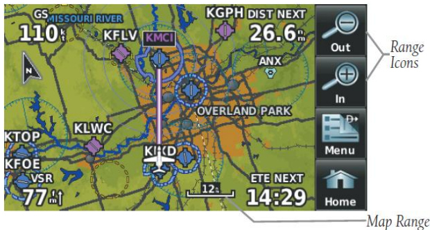
Fig. 7-16 Garmin AERA 500 / 510 map screen (air navigation mode)
