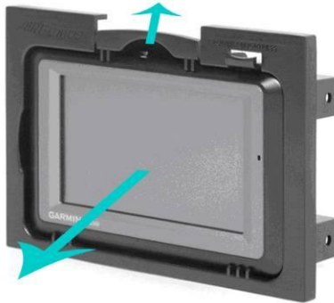
Fig. 7-18 Garmin GPS AERA AirGizmos panel dock
